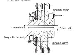
Type 4 When the Torque Limiter is used with a coupling type, and the main unit side stops when overload occurs.
