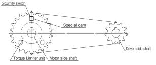
Type2 When the driven side experiences overload, the Torque Limiter unit stops.
