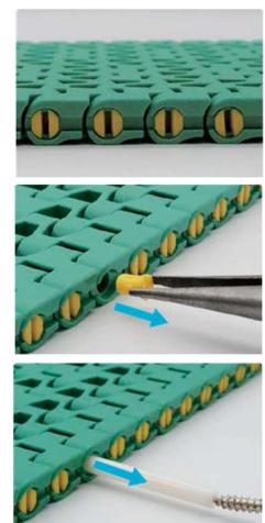
② Using a threaded head screwdriver, screw it into the center hole (1mm diameter) of the pin, and pull out the pin to disassemble the chain.
