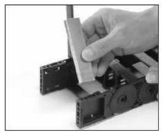
The crossbar of the Universal Mounting Brackets must be opened for assembly and disassembly of the strain relief comb and C-Profile. Fix the strain relief comb or C-Profile into Universal Mounting Brackets and close the crossbar.
