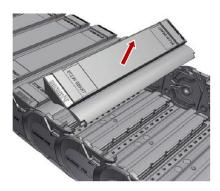
4) Remove the fixed end outside cover (material: resin) and outside bracket cover (material: aluminum) in the same way as 1) and 2) above.
