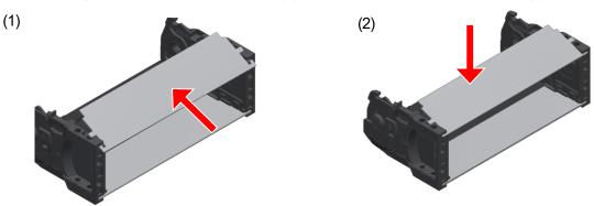
2) Install the fixed end outside cover. Insert the fixed end outside cover in the direction of the red arrow into the indentation on the link circled in the following images, and then tap with a plastic hammer to complete installation.
