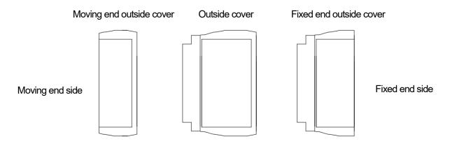
1) Install the bracket covers (material: aluminum) to the moving end and fixed end brackets. After inserting the bracket cover as shown in (1), fit the cover from above as shown in (2).
