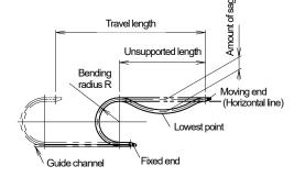
7-7 If the machine will be stored following installation, fix the moving end of the cable carrier so that it is at the end of its reverse stroke to prevent sag in the unsupported length portion due to creeping. Moreover, use supports or some other means to hold the center unsupported length portion if not possible given the system structure.
