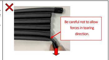
Be sure to fix the device in a bent position with the locking part facing the outside.
