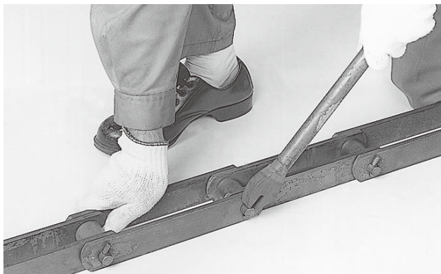
The photo shows a T-pin being bent.
