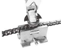
Fig. 2 Grinding the pin ends
