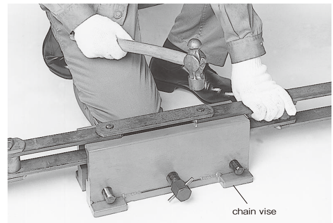
The photo shows a chain vise being used to remove a C-pin.
