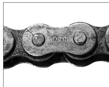
Fig. 35 Hydrogen embrittlement cracking
