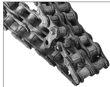
Fig. 34 Corrosion of stainless steel roller chain
