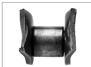
③ Offset link plate fatigue breakage
