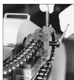
Fig. 5 How to cut a chain using a chain screw1 Rivet-type roller chain
